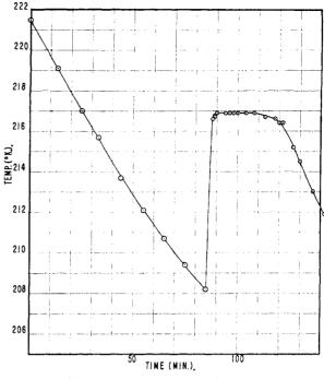
Fig. 3.—Borazole freezing point curve.
