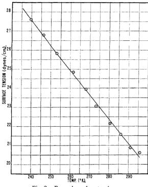
Fig. 2.—Borazole surface tension.
